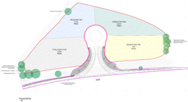
Image 01 – Initial site layout to determine vehicle access and individual areas for development
