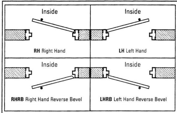
When standing outside, if the door opens toward the right (out of the area), it takes a left hand hinge (also referred to as right hand reverse bevel, RHRB). If it opens to the left, it takes a right hand hinge (also referred to as a left hand reverse bevel, or LHRB). This may be a difficult concept to grasp at first, but do not be discouraged. Just practice during everyday encounters with various openings.
