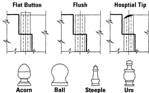
The *flush/concealed tip* is the second most commonly used tip, and this is concealed inside the knuckle. It is often more pleasing to the architect because of the fewer lines across the face of the hinge knuckle.
