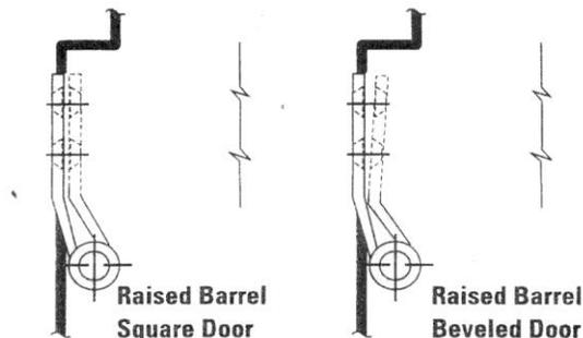
Another special function available is the raised barrel hinge, which is used when the door is set back into the frame. There are three different types of applications: Jamb Surface Mount, Raised Barrel for Square Edged Door and Raised Barrel for Beveled Edge Door. The hinge knuckle is offset to allow it to clear the obstruction of the frame.
