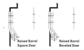
Another special function available is the raised barrel hinge, which is used when the door is set back into the frame. There are there different types of applications: Jamb Surface Mount, Raised Barrel for Square Edged Door and Raised Barrel for Beveled Edge Door. The hinge knuckle is offset to allow it to clear the obstruction of the frame.
