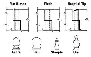
The *flush/concealed tip* is the second most commonly used tip, and this is concealed inside the knuckle. It is often more pleasing to the architect because of the fewer lines across the face of the hinge knuckle.
