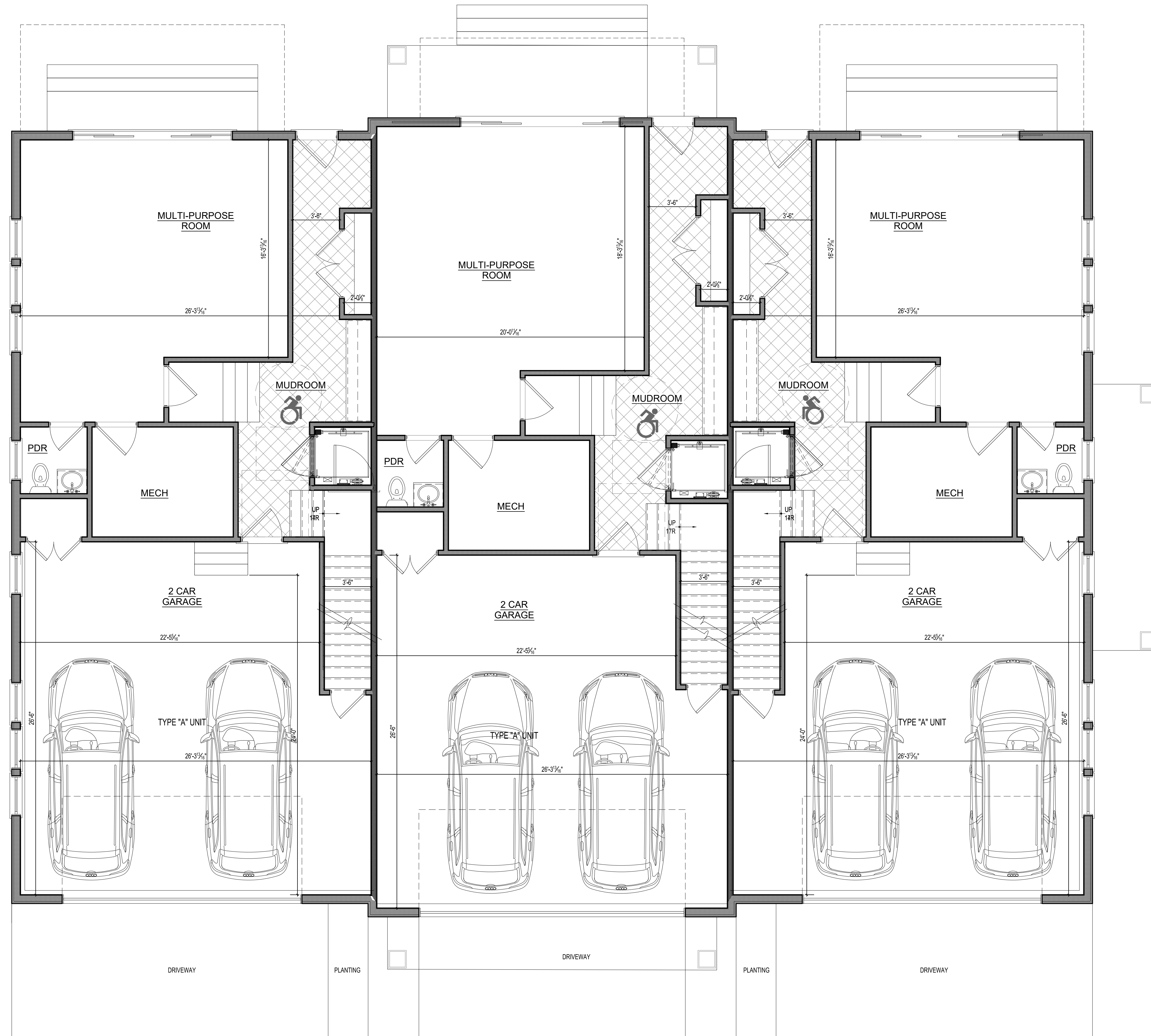
1 BUILDING "C" PLAN: PROPOSED FIRST FLOOR
