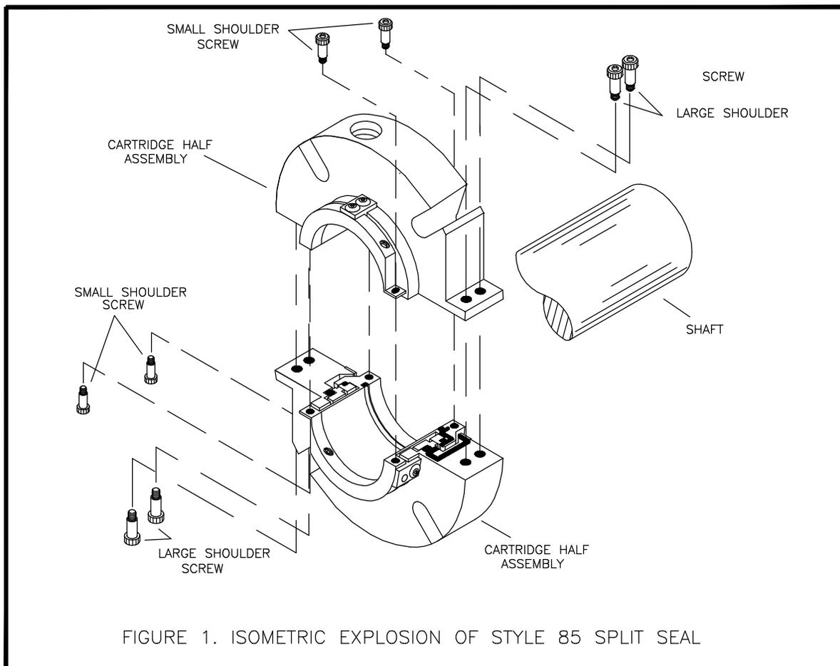
FIGURE 1. ISOMETRIC EXPLOSION OF STYLE 85 SPLIT SEAL
