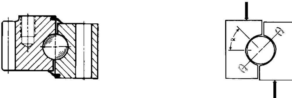
**FIGURE 3—FOUR POINT CONTACT BEARIN GCROSS SECTION**
