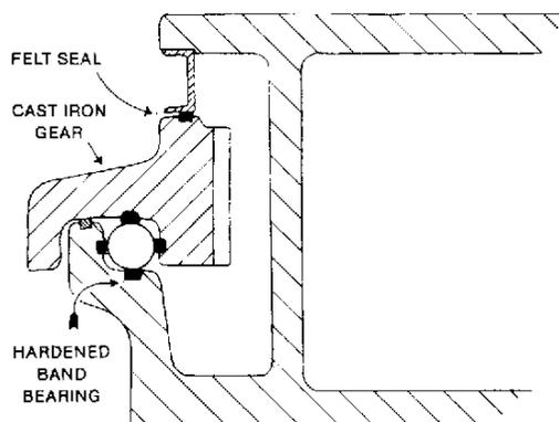
FIGURE 1 - CAST IRON DRIVE WITH INSERTED RACEWAY BEARING
