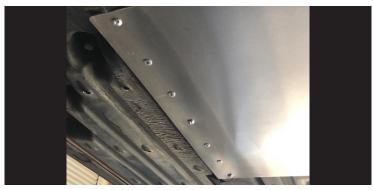
The pre-cut holes in the plate work as a guide to drill the holes that are needed for the correct installation of the provided rivets and security screws. The provided self tapping screws are used in the furthest corner holes to hold the plate in place while drilling the rivet holes. The self tapper can be use to pre-drill holes for the security screws as well.
