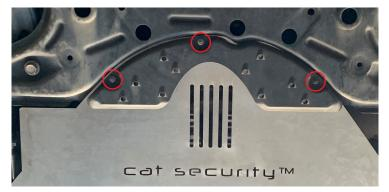
The Cat Security<sup>™</sup> plate is mounted on the front 3 factory studs and the OEM splash guard is installed over the plate. This allows for the plate to be centered and aligned with the frame rails on each side. These nuts are kept loose until all other fasteners are installed. These (3) 10mm nuts should be tightened last.
