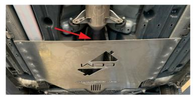
If installed correctly, there should be enough space between the catalytic converter and the Cat Security<sup>™</sup> plate to ensure there are no vibration noises or unwanted contact. After the installation of the security screws and rivets be sure to tighten the front (3) 10mm bolts.
