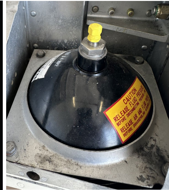
Unfeathering Accumulator 135psi +/- 5 psi Nitrogen
