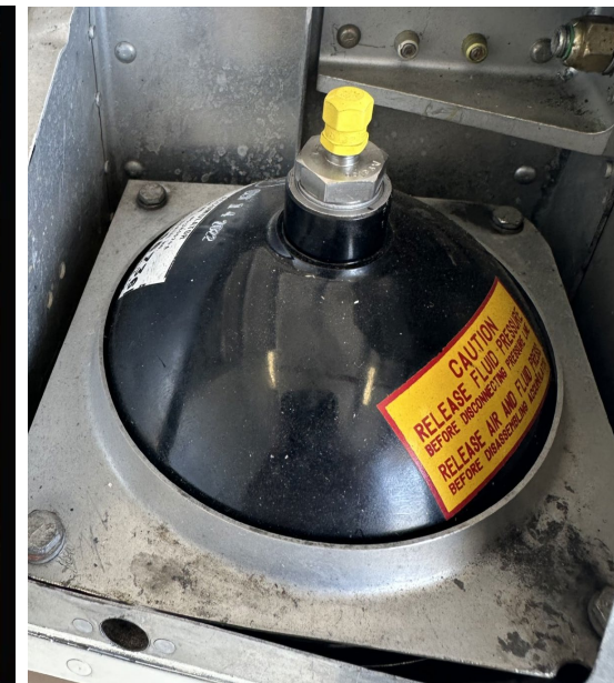
Unfeathering Accumulator 135psi +/- 5 psi Nitrogen
