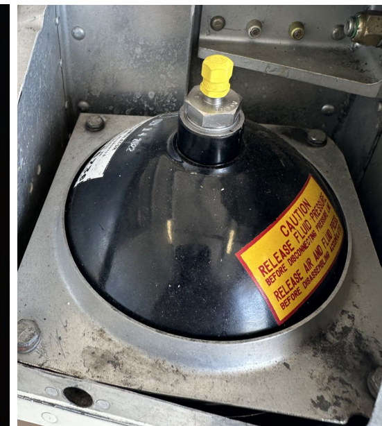
Unfeathering Accumulator 135psi +/- 5 psi Nitrogen
