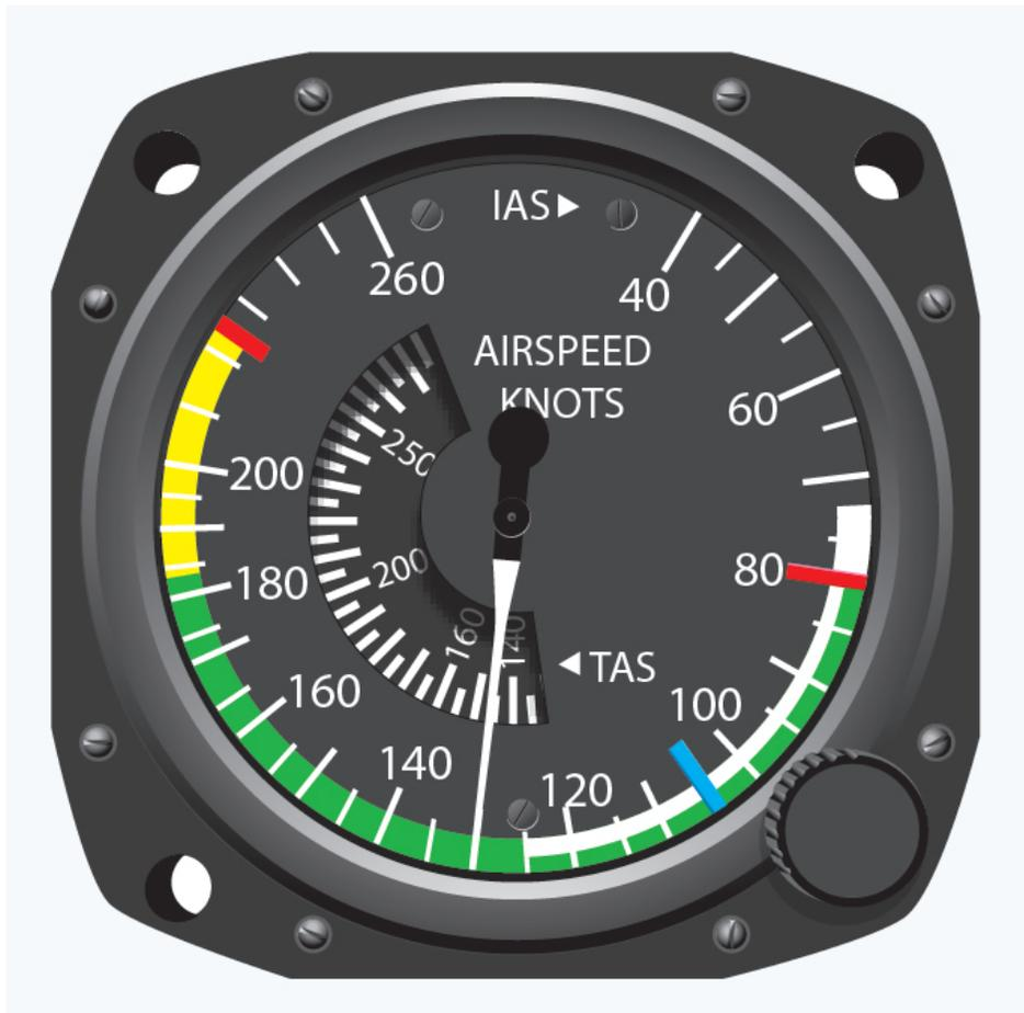
Figure 13-1. Airspeed indicator markings for a multiengine airplane
