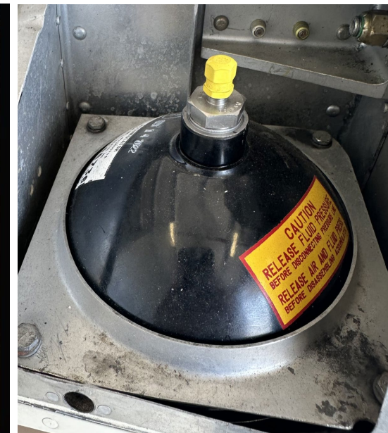
Unfeathering Accumulator 135psi +/- 5 psi Nitrogen
