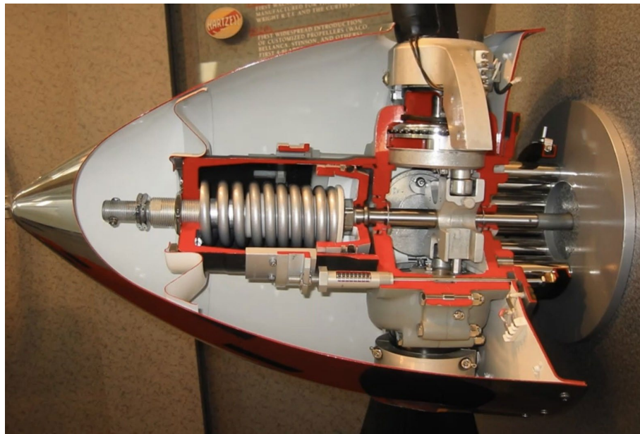
Full-Feathering Propeller – cutaway view
