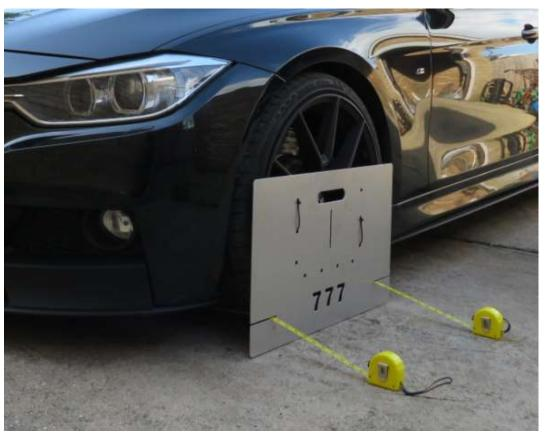
7. Pull the tapes tight and observe the reading at the exact point the tape exits the plate.
