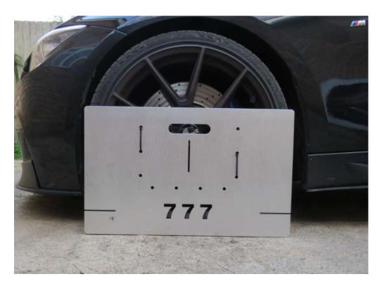
5. Repeat this procedure for the opposite wheel. Check the steering is still straight once complete.
