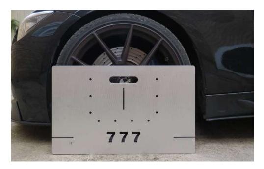
4. Use the holes to cable tie the plate to the wheel. Making sure the plate is still central, is in equal contact with the wheel rim/tyre around its radius and does not deform from excessive cable tie force.
