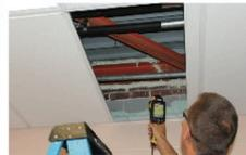
Building components inspected and tested by Canam revealed that gaps and cracks in the schools' building envelopes were allowing air to uncontrollably infiltrate and exfiltrate the building. An analysis of each component revealed that the roof-to-wall intersections were primary leak sources due to original construction.
