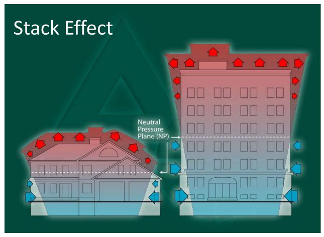
Stack effect is a temperature-driven phenomenon, which is especially noticeable in cold weather, when warmer indoor air, which is more buoyant than the colder outdoor air, tends to rise in the building.
