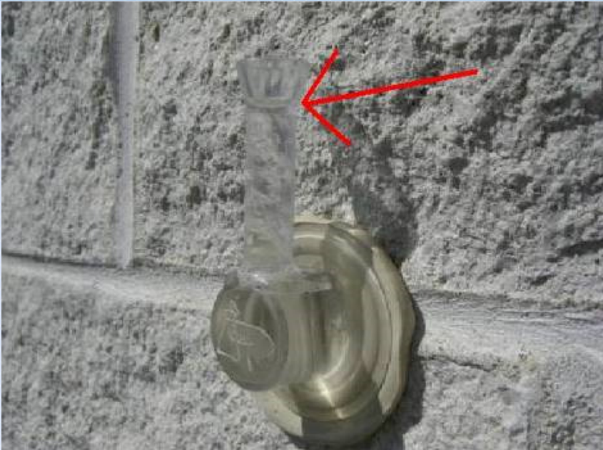
Above: Water-filled RILEM tube at start of test Above: Water 20% absorbed after 5 minutes
