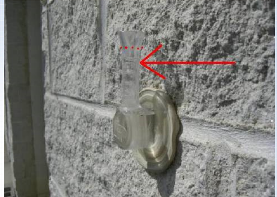
Above: Water-filled RILEM tube at start of test Above: Water 20% absorbed after 5 minutes
