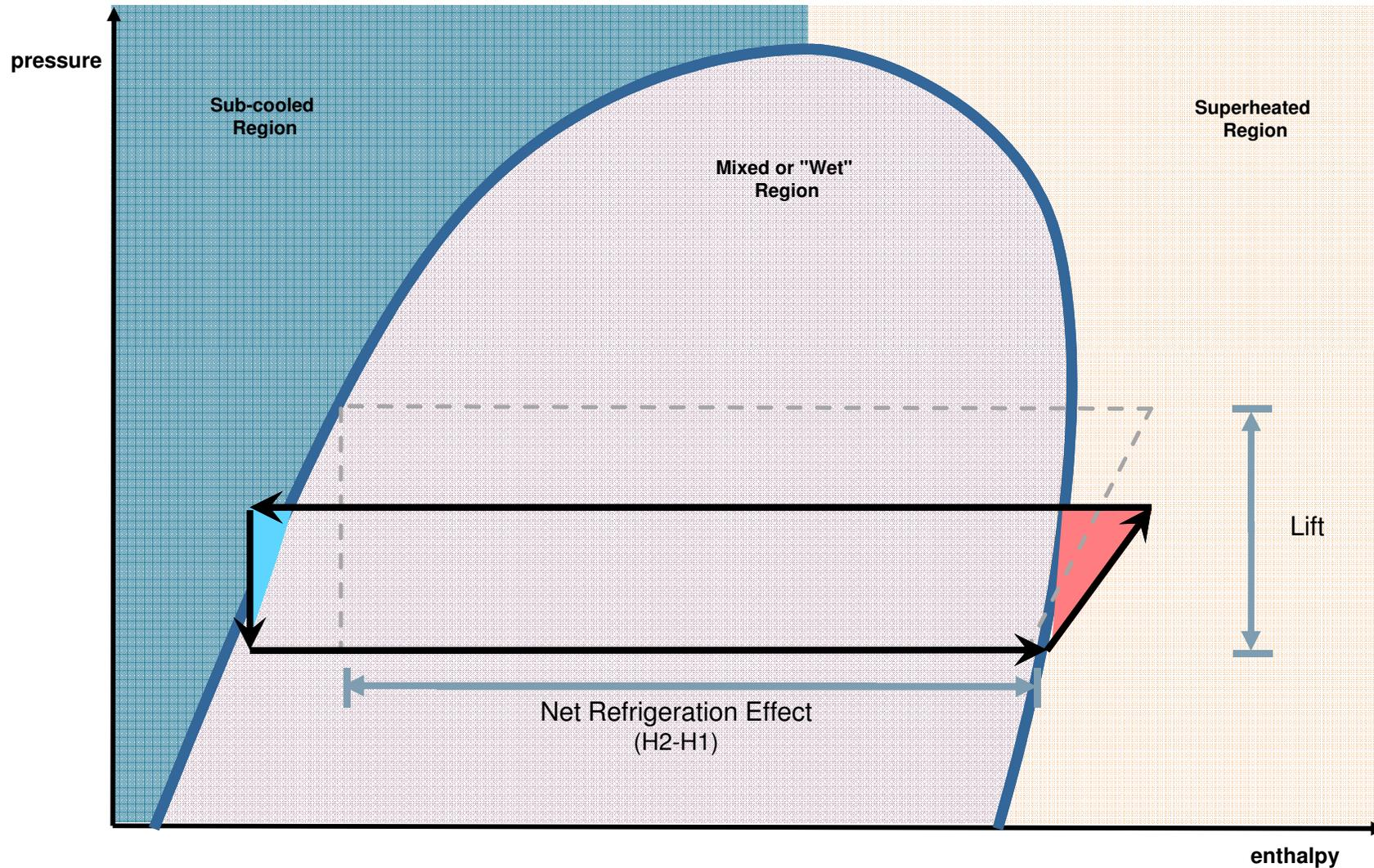
**Compressor Energy = Mass Flow of Refrig. x Differential Pressure or 'Lift'**
