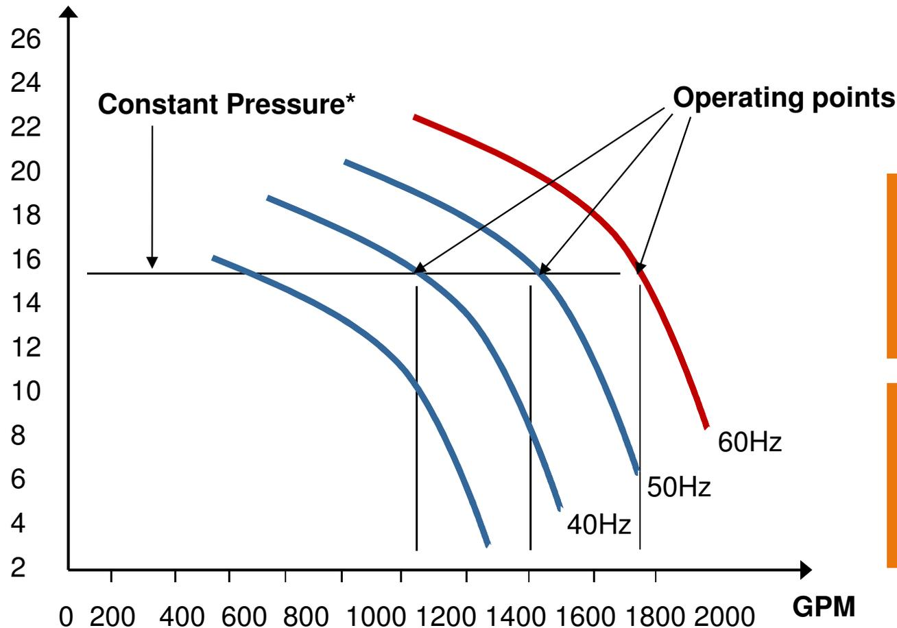
A typical control strategy is to control to a constant differential pressure in the loop
