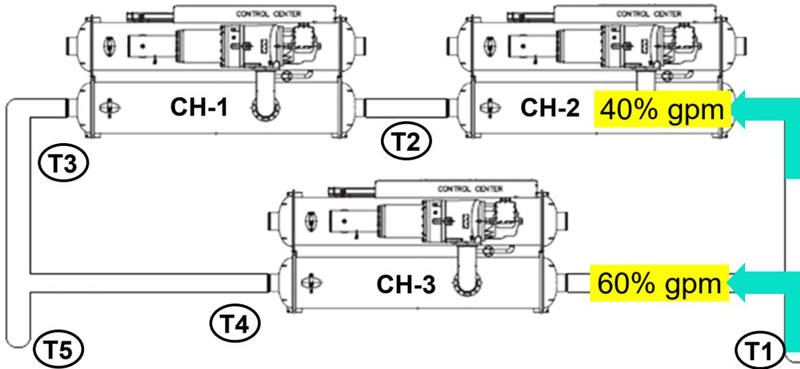
When standby chiller enabled, flow may not be balanced between branches.
