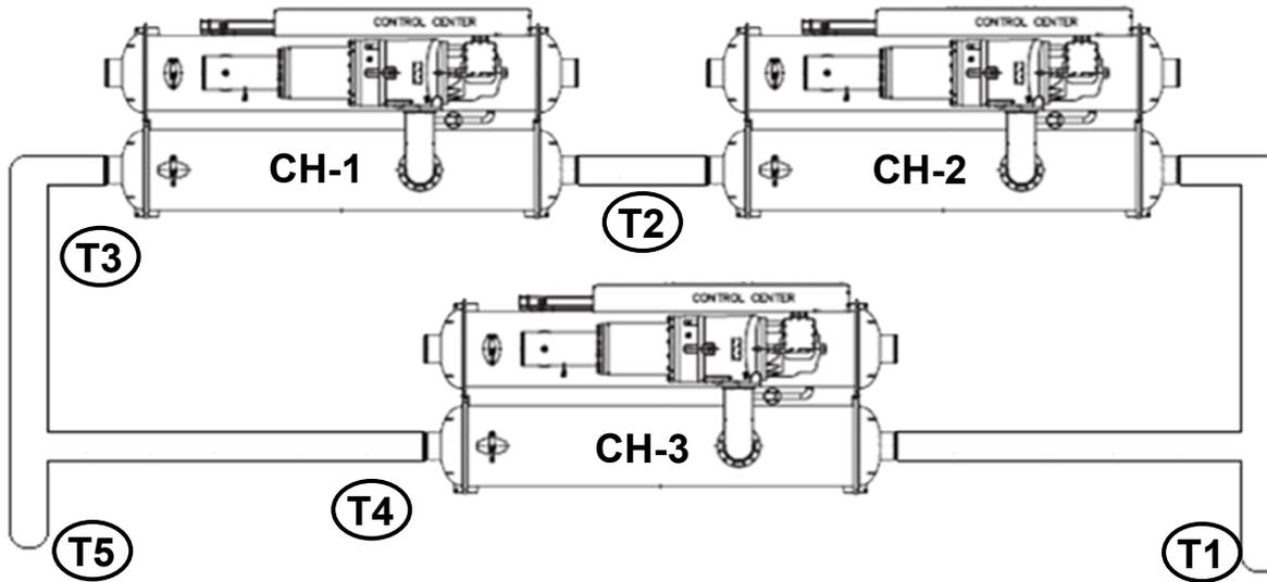
BSM enables LEAD/LAG Chillers (CH-1 and CH-2) as Required to meet T5.
