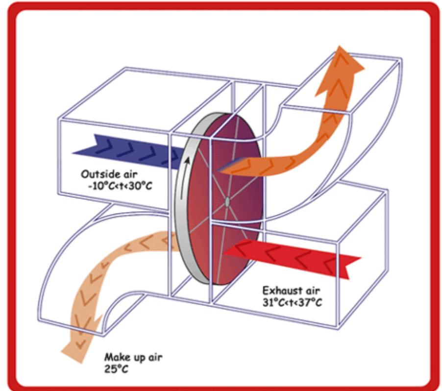
A diagram of a rotary heat exchanger, or "heat wheel"
