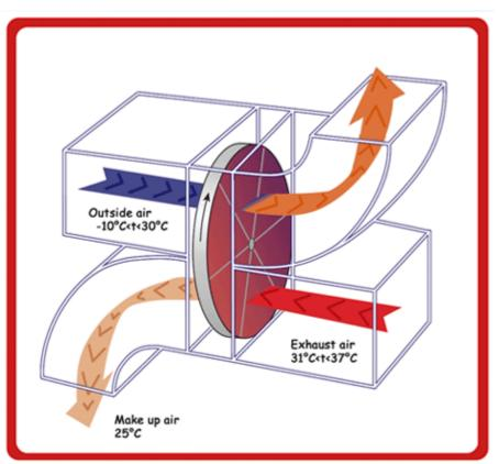
A diagram of a rotary heat exchanger, or "heat wheel"
