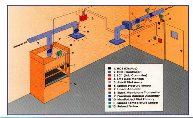
Less Exhausted Air Equals Less Conditioned Intake Air
