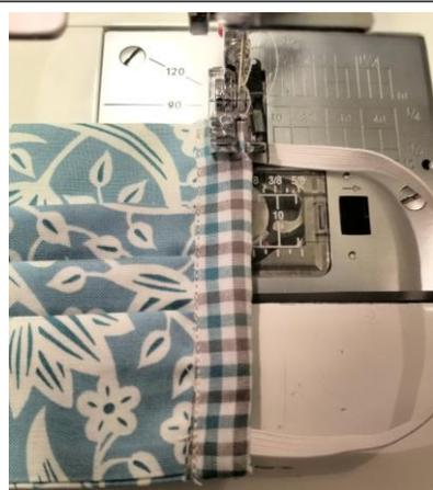
This step isn't necessary. It just gives it a nice finished look and helps to give that elastic a little extra stability. Stitch down the edge of the mask close to the elastic side.
