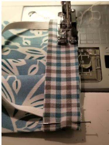
Using a 1/4 inch seam allowance, stitch the length of the entire edge, making sure to back stitch at the beginning and end.
