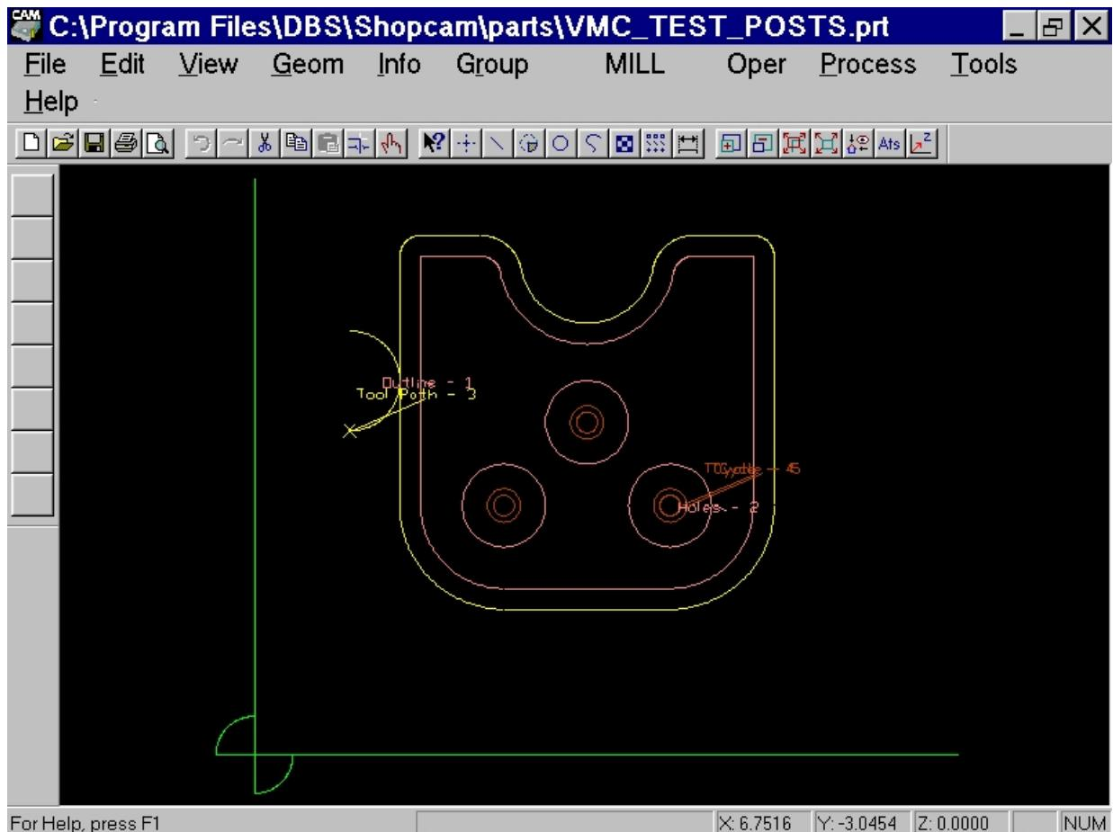
The first operation is a finish pass clockwise around the shape. The endmill positions at X0.573 Y1.95 then rapids to Z0.1 The full depth is Z-.122
