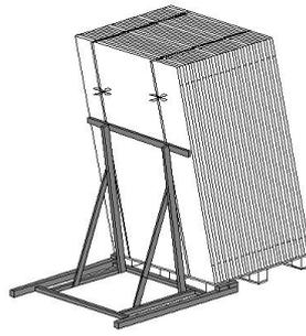
Gently push the assembly so that it leans against the support frame and remove the vertical steel strip
