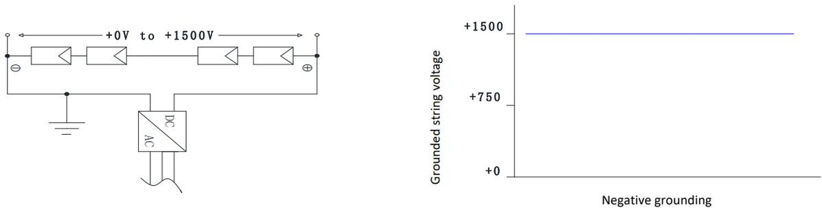
Figure 3. Schematic diagram of grounding potential of inverter
