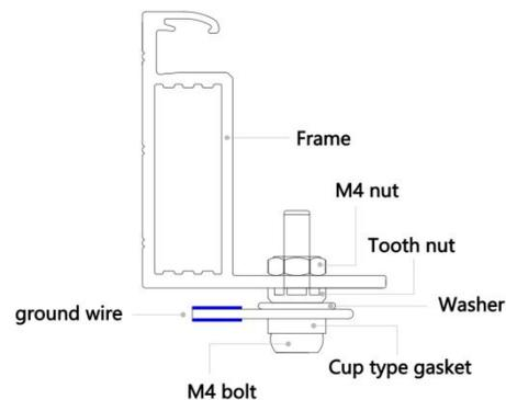
Figure 2. Grounding method
