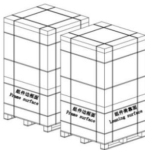
Unpacking the reclining surface needs to be close to a solid wall or another pallet of intact components of the same size
