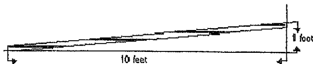
Figure 1: A 10% slope is represented by leaning a board against the wall with the top at 1 foot and the base set 10 feet away from the wall.
