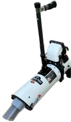
Figure 14 Handle installed for the no-wheels configuration.
