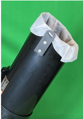
Figure 21: Litter-Vac Bag inserted into canister opening and folded over.
