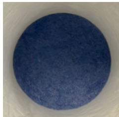
Figure 6: Plastic Mesh Particulate Filter located in front of the Protective Debris Screen.
