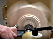
flute to prevent a catch. Rich then began using a shear scrape to refine the wing shape and remove tool marks, using very light pressure as he approached the wing tips.
