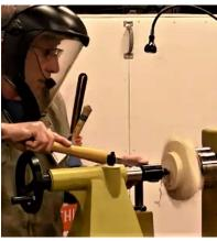
easily. As Rich said, the opening for the chuck jaws doesn't have to be very deep, Depending on the wood, and how aggressive you turn, 1/8 to 1/4" depth is sufficient.
