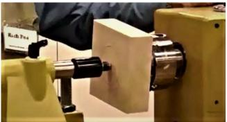
tightened againsst the piece, forming a friction hold against the chuck jaws. Rich only lightly tightens the quill lock, as he will be tightening with the hand wheel frequently to maintain the mounting.
