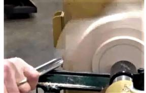
lightly advance the tool into the wood. The distance over the tool rest **does not change**. If it does, you will most assuredly get a catch. You just change the angle of the tool enough to start to cut, with the flute at approximately 45 degrees. Although this change in angle is done with the back hand (locked against your hip, of course), it is very like beginning a cut on a spindle, where you bring the bevel gently against the wood, and then raise the handle until the tool starts to cut.
