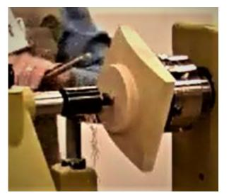
You can see now that the upward curve has been defined. As stated earlier, as you start the cut and proceed, the flute should be approximately 45 degrees to the wood surface. As you approach the end of the cut, you want to close the flute. This both gives a sharp angle between what you are removing and what remains, and it also greatly reduces the potential of a catch.
