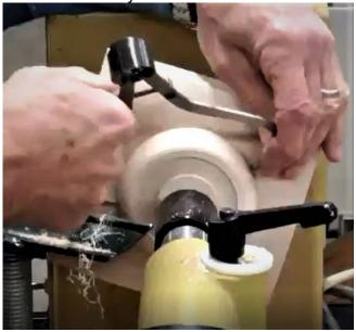
Now it's time to reverse the piece, onto the chuck jaws in expanding mode. Expand the jaws securely into the recess/mortise, being careful not to tighten so much that you break the foot. Oh yes, it really is possible to do that.
