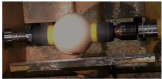
Then change the axis slightly and do it again. As many times as you need to achieve the finished sphere you want. Remember, at each of these axis rotations, you are just taking off the high points and tool marks, not changing the diameter. Sanding can be done at each rotation as well.
