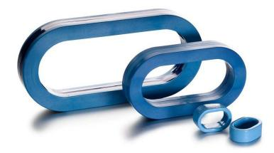
High-frequency common-mode (HF-CM) core kits are one way to reduce bearing wear. They should not be used as the sole mitigation technique. The HF-CM cores work by reducing the high-frequency common-mode currents that are associated with the electric discharges in the bearing. The cores also reduce the high-frequency emissions from the motor cable which can be used in applications with unshielded motor cables.
