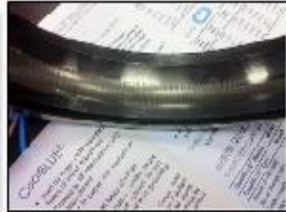
Fluting from Common Mode Currents
