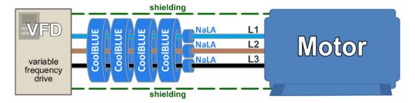
¼ hp to 10hp must have power cables run through CoolBLUE cores twice (two turns) in order to provide enough inductance to properly suppress common mode peak current. NaLA is applicable in all ¼ hp to 10hp motors, and only one turn per NaLA core.
