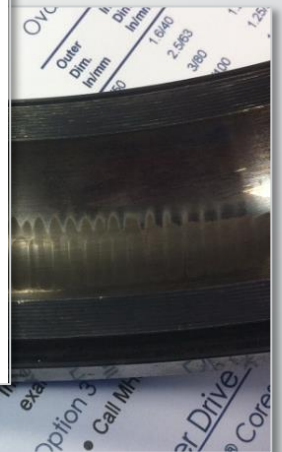
Example: Outer Bearing Race Fluting EDM Results from VFD Induced Common Mode Noise
