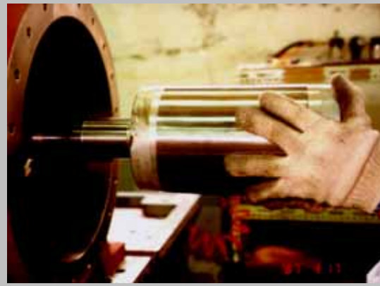
圖 Figure 2-8 拉出馬達轉部/ Pull the motor rotor out.
