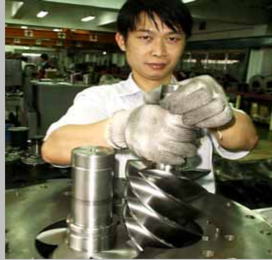
圖 Figure 3-2 母轉子組裝 Female rotor assembly.
