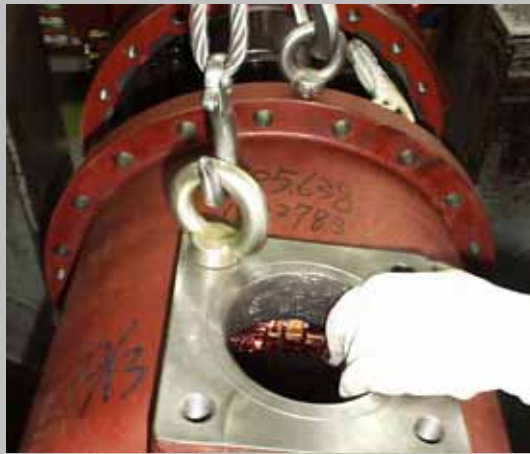
圖 Figure 2-6-3 SR-4(H)~8(H) 拆解馬達外殼/ Take Apart Motor Cover & Motor Casing
