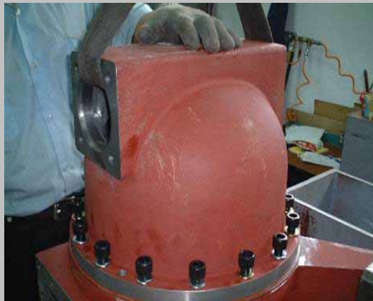
圖 Figure 2-6-2 SR-434 拆解馬達外殼/ Take Apart Motor Cover & Motor Casing
