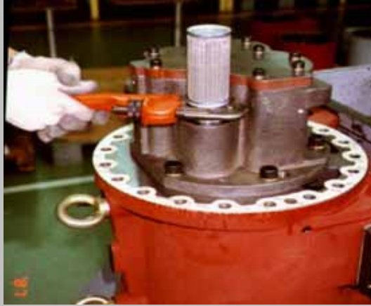
圖 Figure 2-9 拆解排氣消音器/ Take out silencer.
