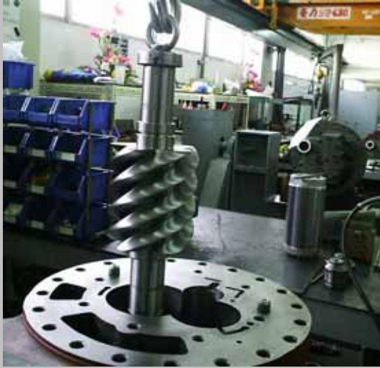
圖 Figure 3-1 公轉子組裝 Male rotor assembly.
