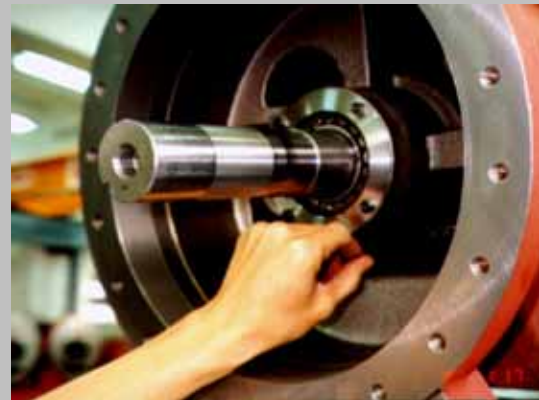
圖 Figure 3-19 固定轉子軸承/ Fix the rotor bearing.
