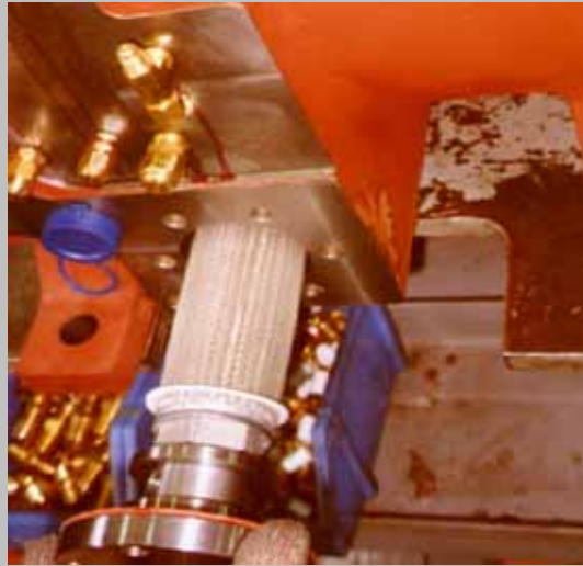
圖 Figure 2-16 拆解機油過濾器/ Take apart the oil filter.
