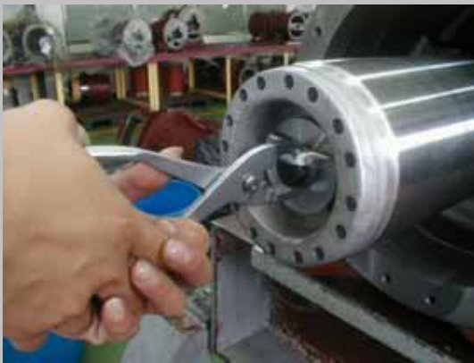
圖 Figure 2-7 取下華司/ Take out the washer.
