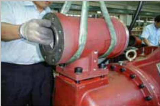
圖 Figure 2-5-1 進氣濾清器拆解 SR-4~7/ Take Apart Suction Filter SR-4~7
