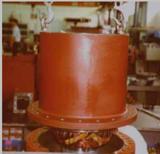
圖 Figure 2-6-1 SR-1(H)~3(H) 拆解馬達外殼/ Take Apart Motor Cover & Motor Casing
