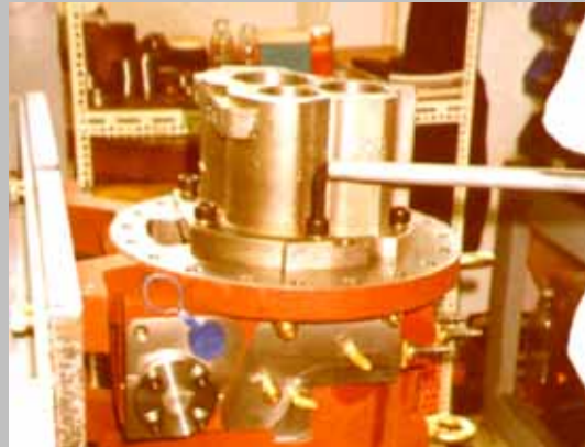
圖 Figure 2-13 拆解軸承座 Take apart bearing seat.
