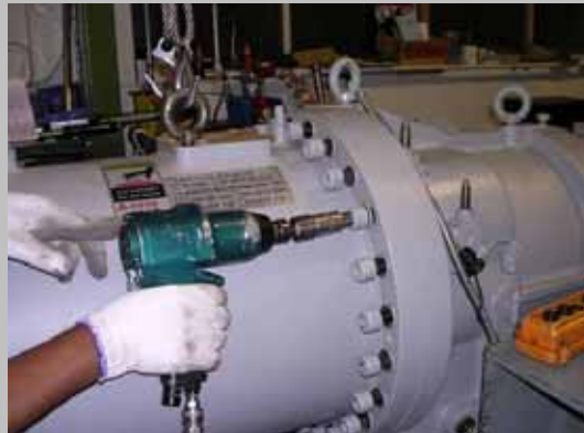
圖 Figure 2-4 油分離器拆解 Take Apart Oil Separator
