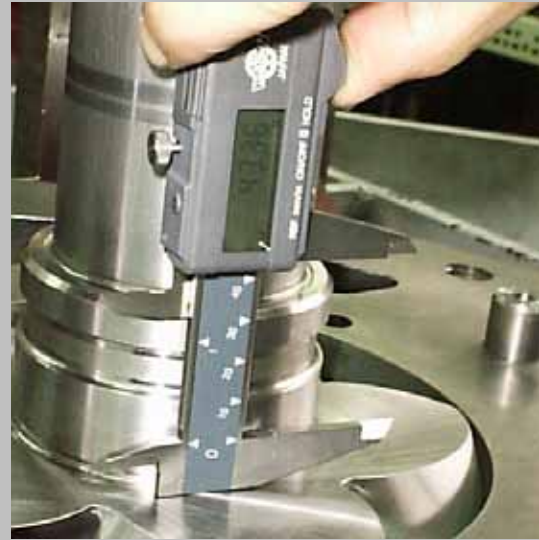
圖 Figure 3-4 量測轉子軸頸長度/ Measure the length of the rotor journal
