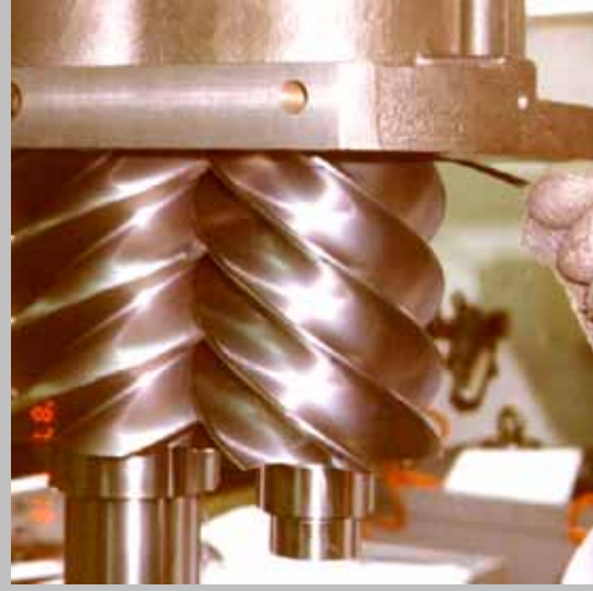
圖 Figure 3-12 量測母轉子排氣間隙/ Measure female rotor clearance.
