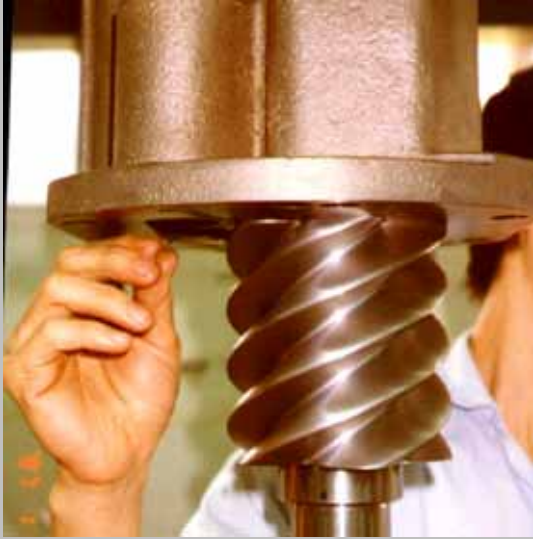
圖 Figure 3-11 量測公轉子排氣間隙/ Measure male rotor clearance
