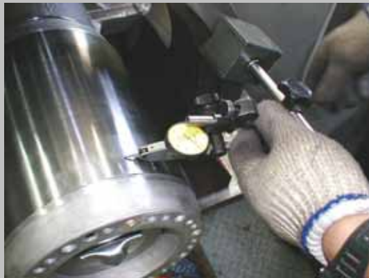
圖 Figure 3-22 量測馬達轉部同心度/ Measure eccentricity of the motor rotor.
