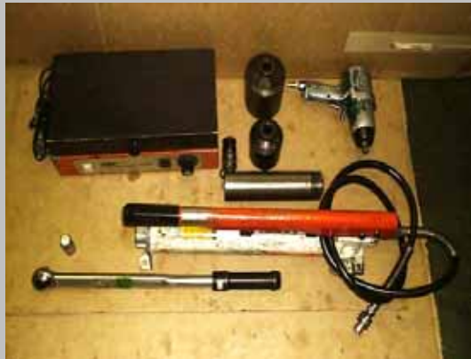
圖 Figure 2-15 拆解軸承座上的軸承/ Take apart bearings on the bearing seat.
