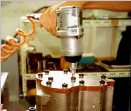
圖 Figure 2-10 拆解軸承座蓋板/ Take apart bearing seat cover.
