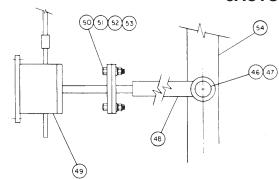
46 PIN F1004306 47 COTTER PIN 48 CLEVIS F10031508 49 JACTUATOR F100653 50 BOLT 1/4-20 x 1.25 F10032310 51 NUT ½-20 F10032403 52 WASHER ½ F10044603 53 LOCKWASHER 1/4 F10044703 54 BAR F201092
