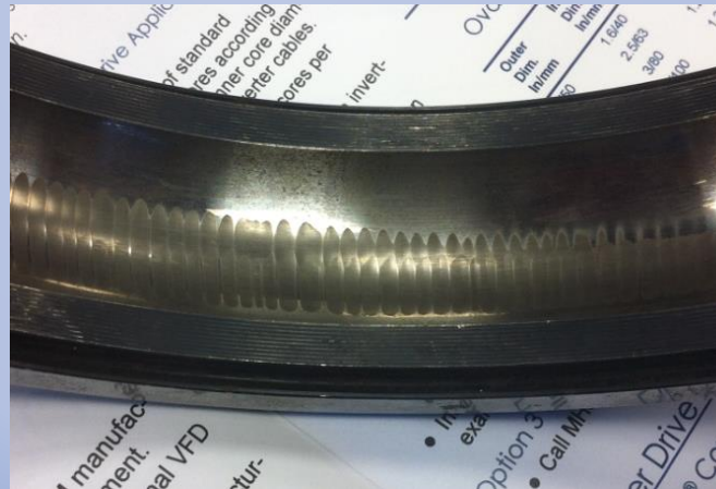
Example: Outer Bearing Race Fluting EDM Results from VFD Induced Common Mode Noise
