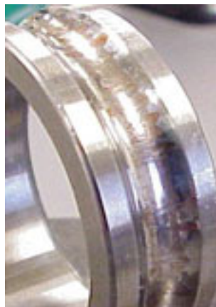
Figure A2-4: Bearing damage from running after false brinelling.
