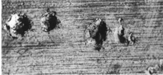
Figure 12: Fusion craters in a bearing race from Scanning Electron Microscope image.
