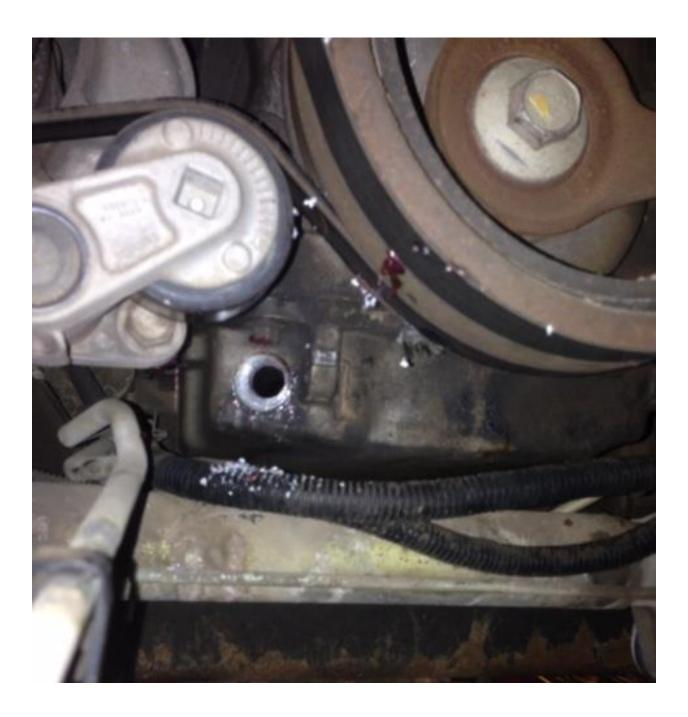
It is important to clean all the metal and grease out of the threaded hole and inside the pan.
