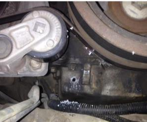
Continue to step up your drill bit size up until you get to the proper 37/64 for the 3/8NPT tap. All drill bits need some type of stop so you do not plunge to deep. (we use 3 sizes when doing this job and grease on the drill bits. Grease is always used when drilling through or tapping the oil pan on the vehicle.
