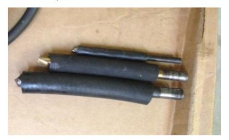
Here is a pic of the drills we use when doing this. The largest drill bit is the proper size 37/64. Notice the rubber hose almost covers the drill bit completely. When installing your drill bit into the drill the rubber hose must cover the entire area and be against the chuck. OR it will not act like a stop
