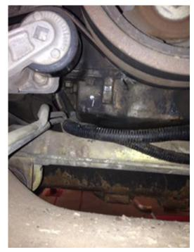
Drill a small pilot hole using a rubber hose to act as stop so you do not punch all the way through.
