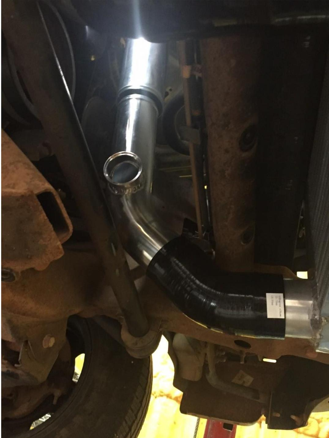
Now if your vehicle is a **99-08 mass air system kit**. You will install the 3-3.750 transition silicone on to the end of your bov pipe. Then your Mass air meter, and finally the 3.750-3.5" transition silicone. If you are using Speed Density tuning, or a 09+ mass air meter. You would install a 3.0-3.5 transition on this BOV pipe.
