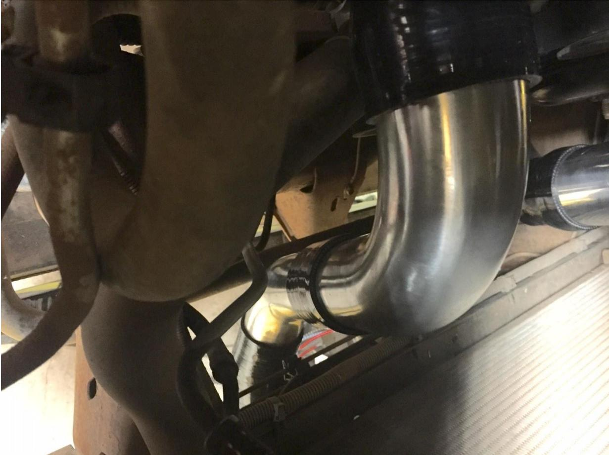
Traveling down, Next will be a Straight silicone and Long leg of 45' aluminum. The end of this 45' aluminum tubing will have a 45' silicone coupler that will attach directly to the inter cooler on the passenger side.
