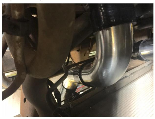
Traveling down, Next will be a Straight silicone and Long leg of 45' aluminum. The end of this 45' aluminum tubing will have a 45' silcone coupler that will attach directly to the inter cooler on the passenger side.
