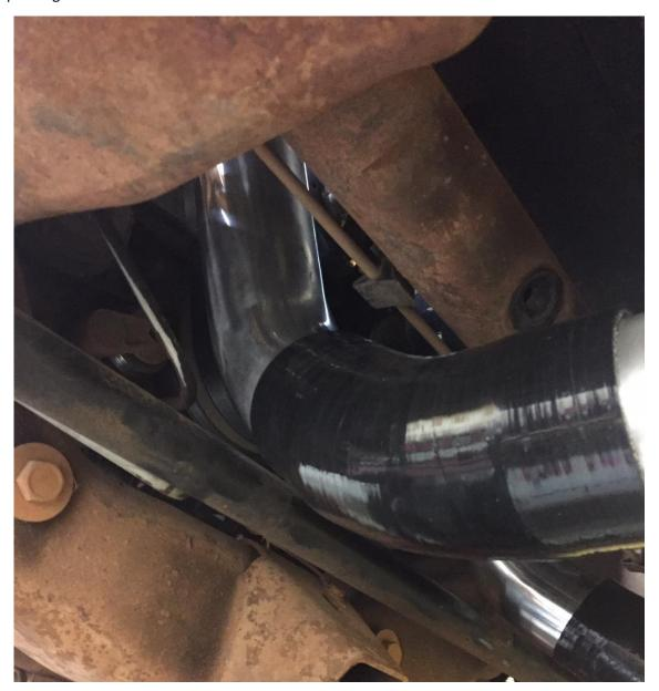
Now tighten the T-bolt clamps on the piping installed. And remember to tighten the compressor cover bolts once finally adjustment is made. The passenger side inter cooler piping routing is completed.
