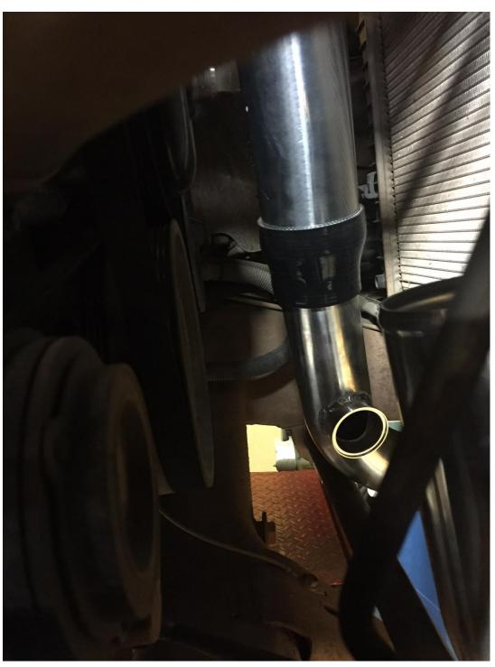
Last aluminum pipe is your 3.5" throttle pipe. The Long Leg will slip in to the 3.5" silicone that was attached to the mass air meter or the BOV pipe directly. The short leg will be aiming at your throttle
