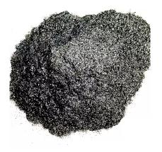
Natural graphite processed by GS technology is a material with distinctively high values of electrical conductivity and has high reflective properties in the infrared thermal range.
