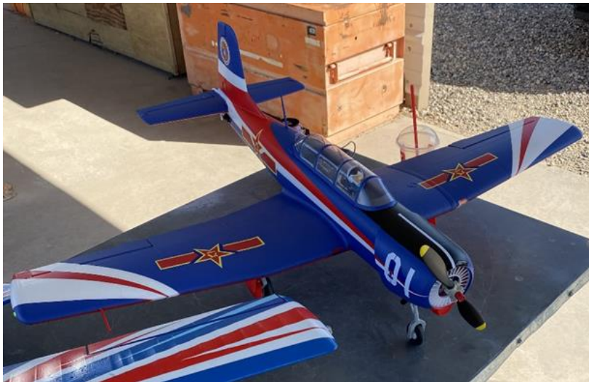
Left, Steve's Yak 130 is a FreeWing model. It has a 70mm motor.
