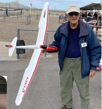
The Moa series are popular balsa kits for r/c sailplanes. The specimen below has a 183-inch span.
