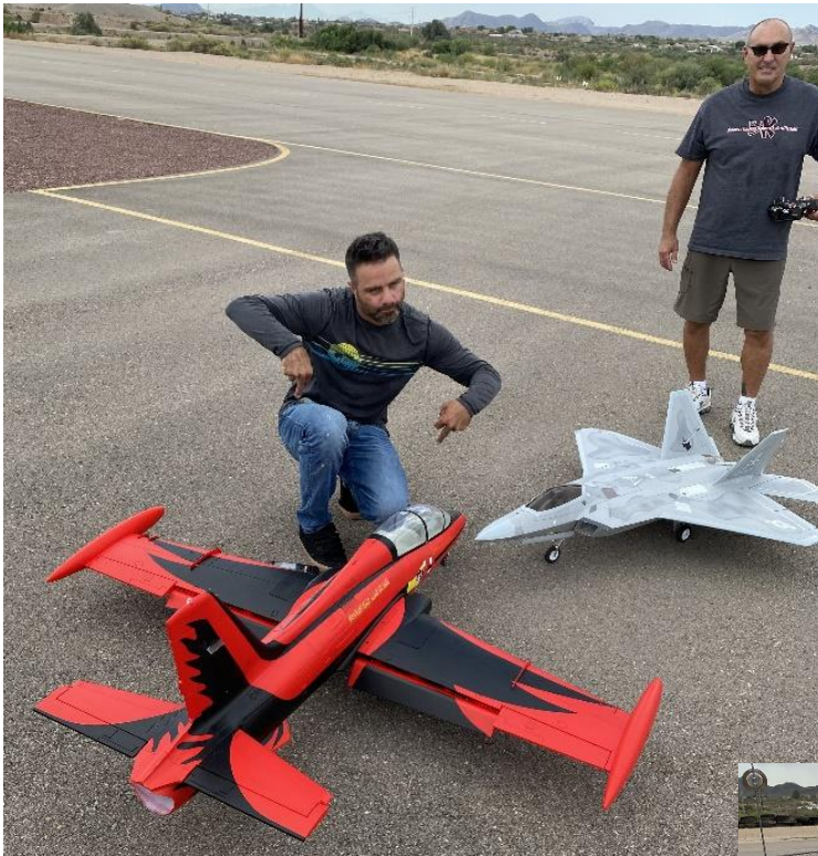
Nick Tocco's AeroFoil Red Dragon Aermacchi MB-339 has a 105mm fan. The wingspan is 63 inches. It weighs 15.9 pounds!
