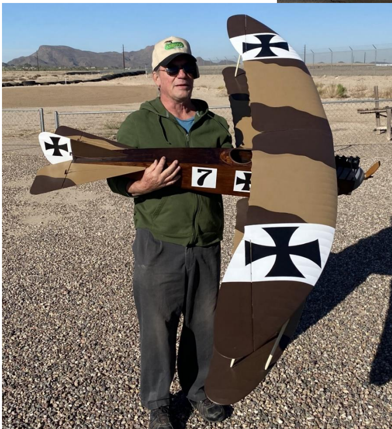
Left, Keith Koppos has produced another masterpiece. This is actually a pre-WWI aircraft. It's a DFW B.I. It has banana-shaped wing that's also double-tapered.
