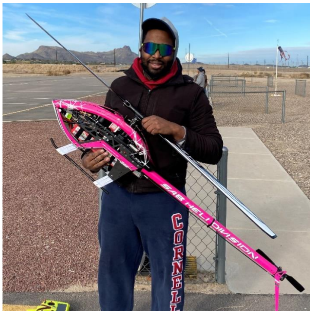
Casey Harris has a new hot pink Goblin 700-size helicopter. That means the main rotor blades are about 700mm long. This is an electric.
