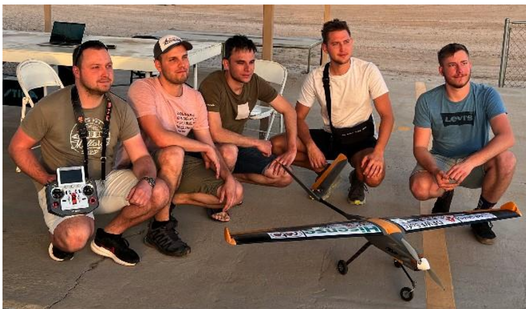
Slovenia University, with a good-looking plane. Double-tapered wings, single motor, winglets, boom empennage, and a v-tail. A mature design.
