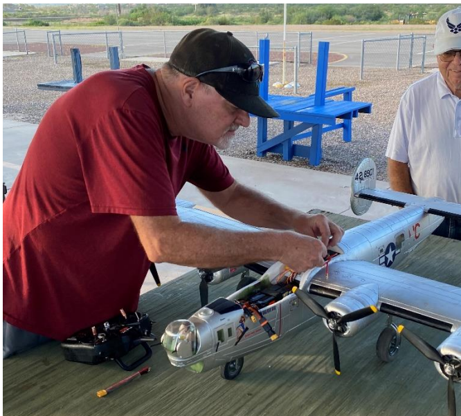
Left, Phil fiddles with a dizzying tangle of wires. Four motors, four ESCs, plus turret servos make for a lot of wire. Phil has simplified things, so some of the functions are inoperative.
