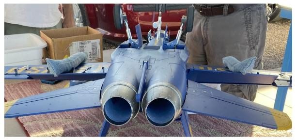
Above, Doug Allen's F-18 developed a severe roll when he deployed the flaps. For a while, Doug worked around the problem by landing with no flaps, and deploying full flaps only on the ground to reduce landing rollout.
