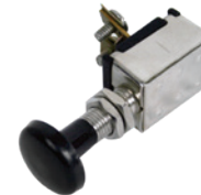
A-L5007 Light Switch, Universal, Heavy Duty Amperage: 20 Position: 2 Terminal: 2 Thread: 3/8" Mounting Stem Type: Push / Pull
