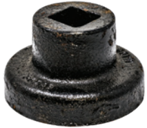
A-VLH6708 Spool Spacer 2-3/8" For 1" Axle, Cast Iron, Painted Black A: 4" B: 2.375" C: 2.250" D: 1.125"
