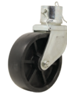
A-VLA2057 Detachable Caster 1000 LB static load capacity 6"x2" reinforced poly wheel zinc plated
