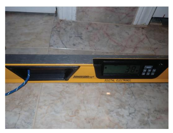
Photo #21 – Unit 3442: Floor sloping up to garage entry, wall finishes/tile cut to fit.
